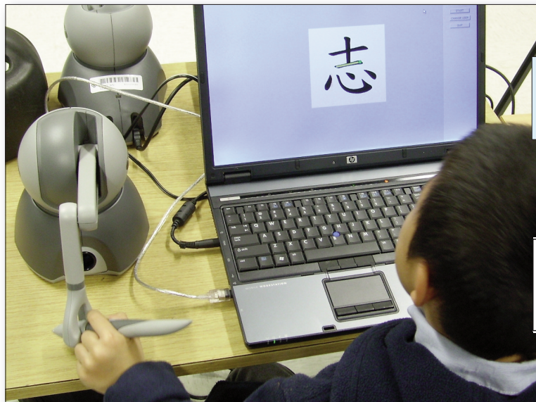
Figure 1 (left): System set-up: the child is holding the haptic stylus to practice handwriting.
